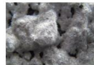
Picture 1 Cold plastic agglomerate road marking after 8 years in service under traffic and snowplow operation at German test field at federal road B4 at Torfhaus (sample 80; applied 30/08/2007)
